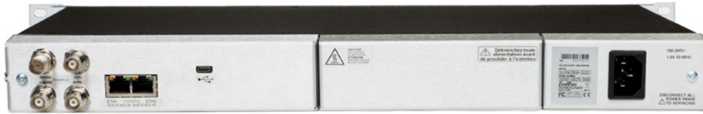
Sonoma rear panel with single power supply (dual AC and DC power supplies available). Two gigabit Ethernet ports. Antenna input TNC connector on upper left. USB Micro-B serial port. Three spare BNC connectors for optional hardware outputs on left.
