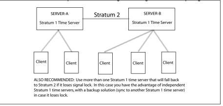
Configuring for Stratum 2 operation is simple and described in the Stratum 2 Product Note. Briefly, you must point Stratum 1 Server-A (for example) to Stratum 1 Server-B by editing the *ntp.conf* file of Server-A and adding a line such as this:
