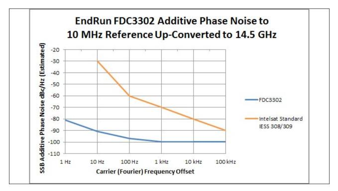
Figure 3. FDC3302 Additive Phase Noise vs. the Intelsat Standard
