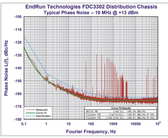
Figure 2. FDC3302 Typical Additive Phase Noise to 10 MHz Signal
