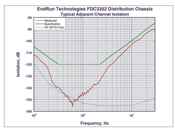
Figure 4. FDC3302 Output Channel Isolation
