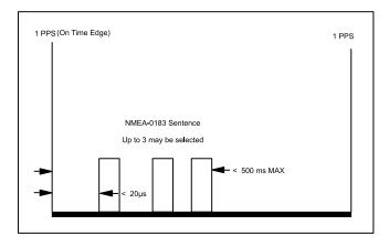
NOTES: If the GPS Receiver is tracking less than 3 satellites then there will be no valid fixes. Therefore, the sentences will be blank. For example: \$GPGLL,,,,,V,N\*64.
