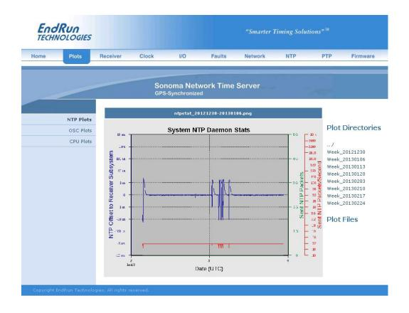
There are four types of data plots available for viewing: CPU, NTP, Oscillator and Receiver. The large data plot shown on any of the plot pages is the last data plot viewed. This could be from any one of the four data types.
