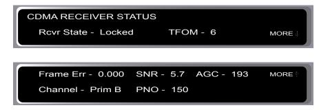
Receiver State: This shows the current state of the CDMA Subsystem. The state may be: acquire, detect, locking, tracking, or locked. When locked, the CDMA receiver is synchronized to the signal and it is disciplining the internal oscillator to remove frequency and time errors.
