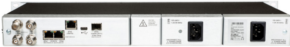
Sonoma D24/N24 rear panel with dual AC/AC power supplies (DC power supplies available). Three gigabit Ethernet ports and a 10 GbE SFP+ port (interfaces to an active optical cable). Antenna input TNC connector on upper left. USB Micro-B serial port. Three spare BNC connectors for optional hardware outputs on left.
