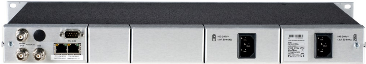
Sonoma rear panel with optional dual power supplies. Antenna input TNC connector on upper left. Two spare BNC connectors on lower left. One RS-232 connector. Two 10/100/1000 Base-T Ethernet ports. Optional dual power supply connectors on right.
