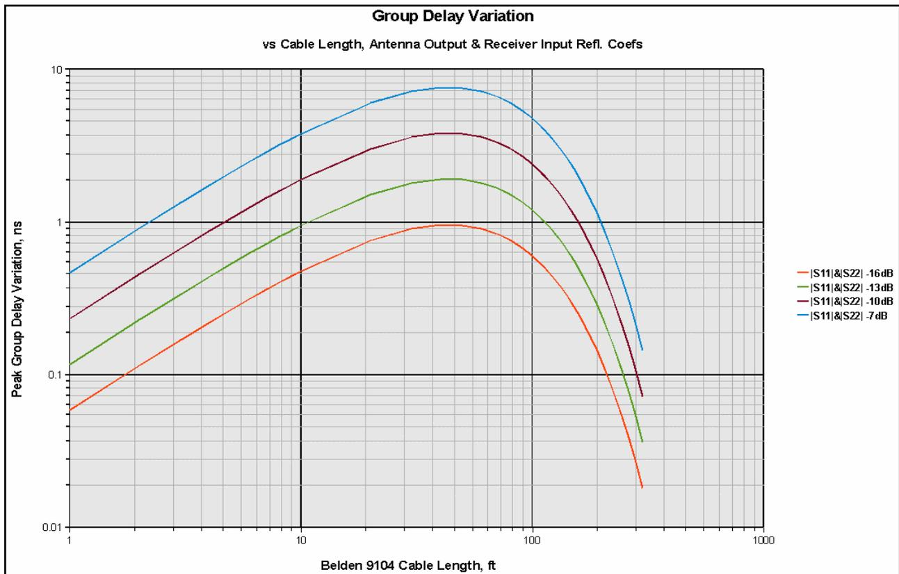
Figure 8. Antenna Download Cable Group Delay Variation Due to Mismatch
