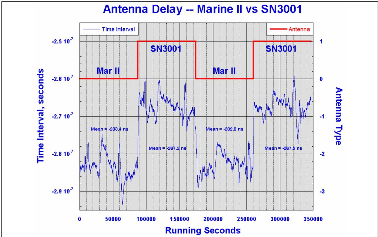
Figure 9. Experimental Verification of VNA Measured Antenna Group Delays
