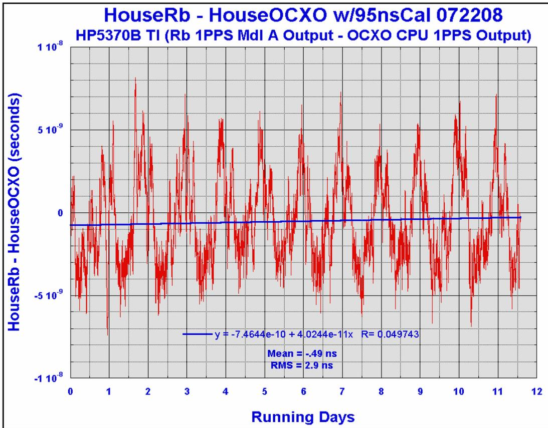
Figure 5. Time Difference Data Between the NIST-Characterized Meridian and a Meridian with OCXO
