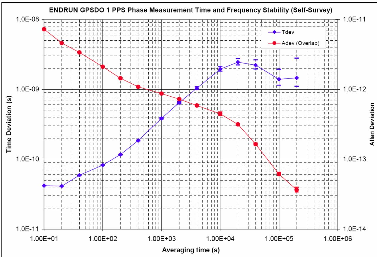
Figure 3. Time Deviation Statistic in Self-Survey Mode
