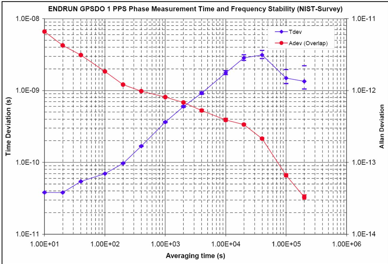
Figure 4. Time Deviation Statistic in NIST Geodetic Survey Mode
