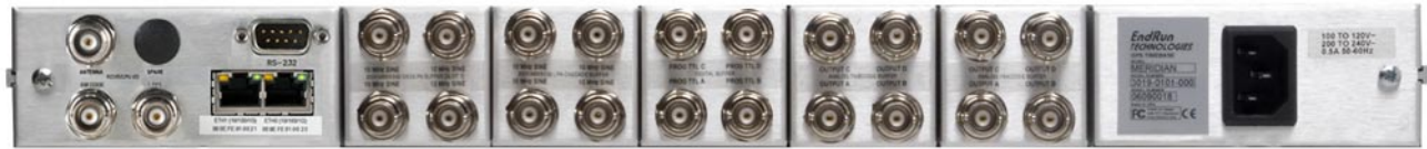
Meridian/Tycho II Rear Panel with Five Option Modules Installed.
