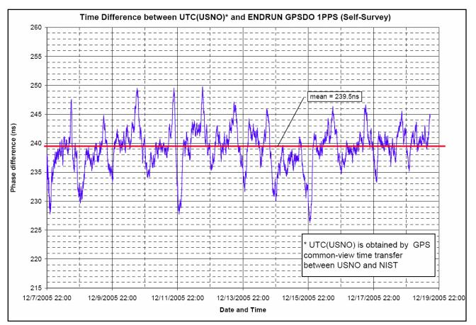
Figure 1. Time Difference Data in Self-Survey Mode
