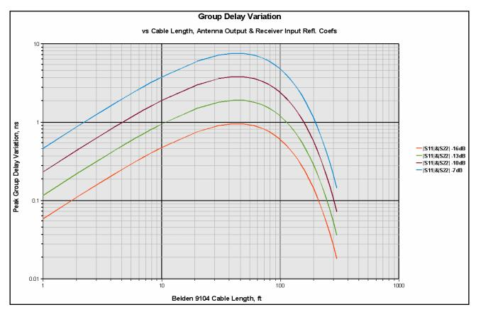
Figure 8. Antenna Downlead Cable Group Delay Variation Due to Mismatch
