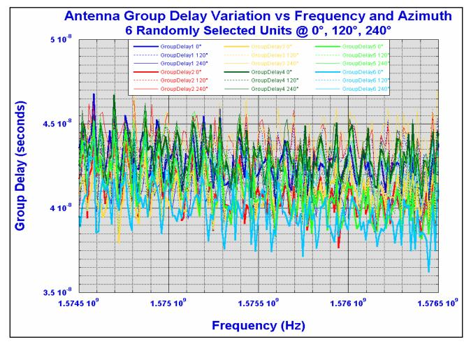
Figure 7. Antenna Group Delay Variation--6 Different Units Measured at 30° Elevation, Multiple Azimuths
