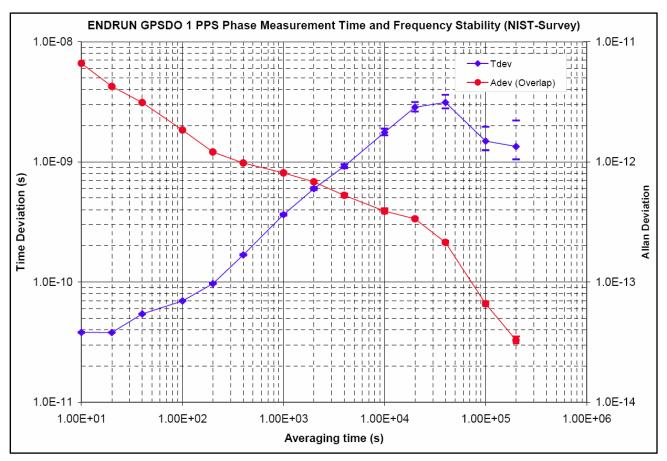
Figure 4. Time Deviation Statistic in NIST Geodetic Survey Mode
