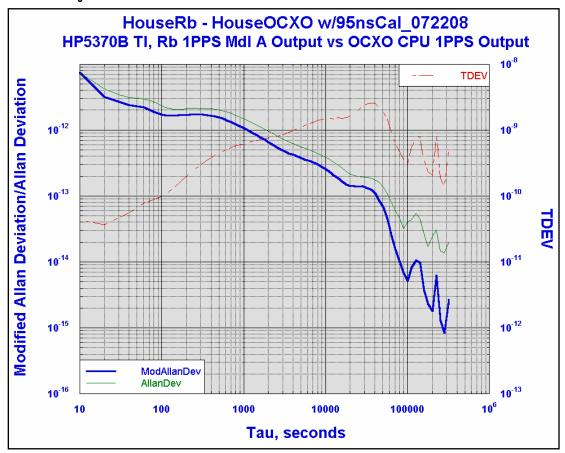
Figure 6. Modified Allan Deviation, Allan Deviation and Time Deviation of the Time Difference Data
