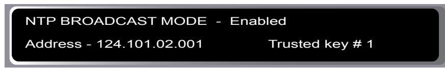
This display provides the user with a convenient means of checking the current configuration and allows limited setup. You may also perform a more complete broadcast/multicast configuration via a **telnet** or **ssh** session or the local RS-232 console using the **ntpconfig** utility. This utility provides a more secure means of setup and is more complete. It will allow you to create keys and identify trusted keys.
