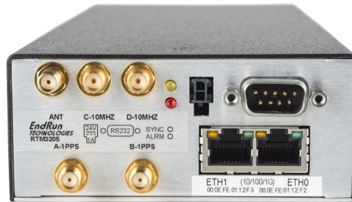
The front panel of a fully-optional RTM3205 with (from left to right): - GPS Antenna Input, Output C - 10 MHz LPN, Output D - 10 MHz LPN (top row SMA connectors) - Output A - 1PPS, Output B - 1PPS (bottom row SMA connectors)
