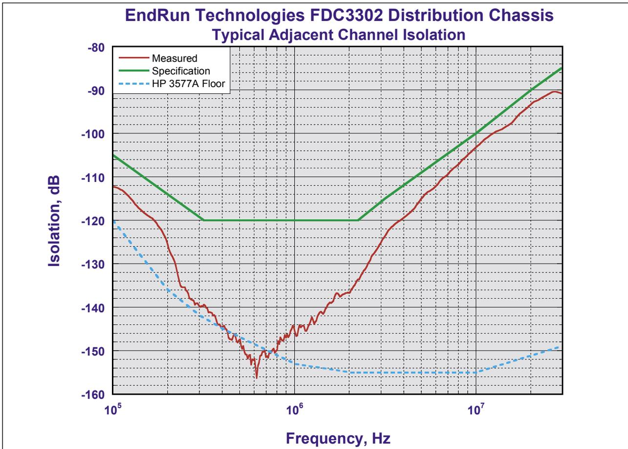
Figure 4. FDC3302 Output Channel Isolation
