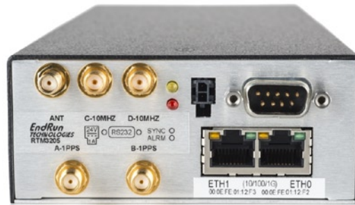
The front panel of a fully-optioned RTM3205 with (from left to right): - GPS Antenna Input, Output C - 10 MHz LPN, Output D - 10 MHz LPN (top row SMA connectors) - Output A - 1PPS, Output B - 1PPS (bottom row SMA connectors)
